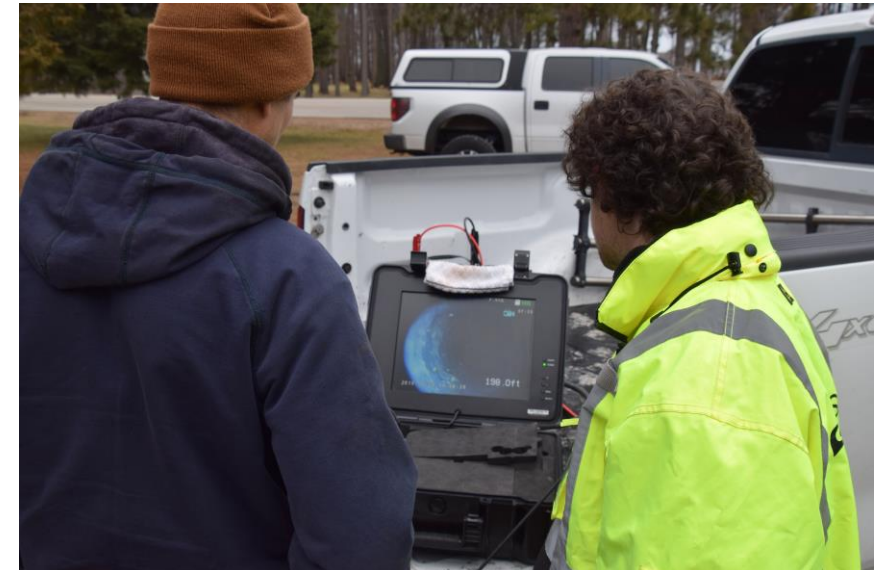
Use camera to quality check well and measure depth; confirm geology
